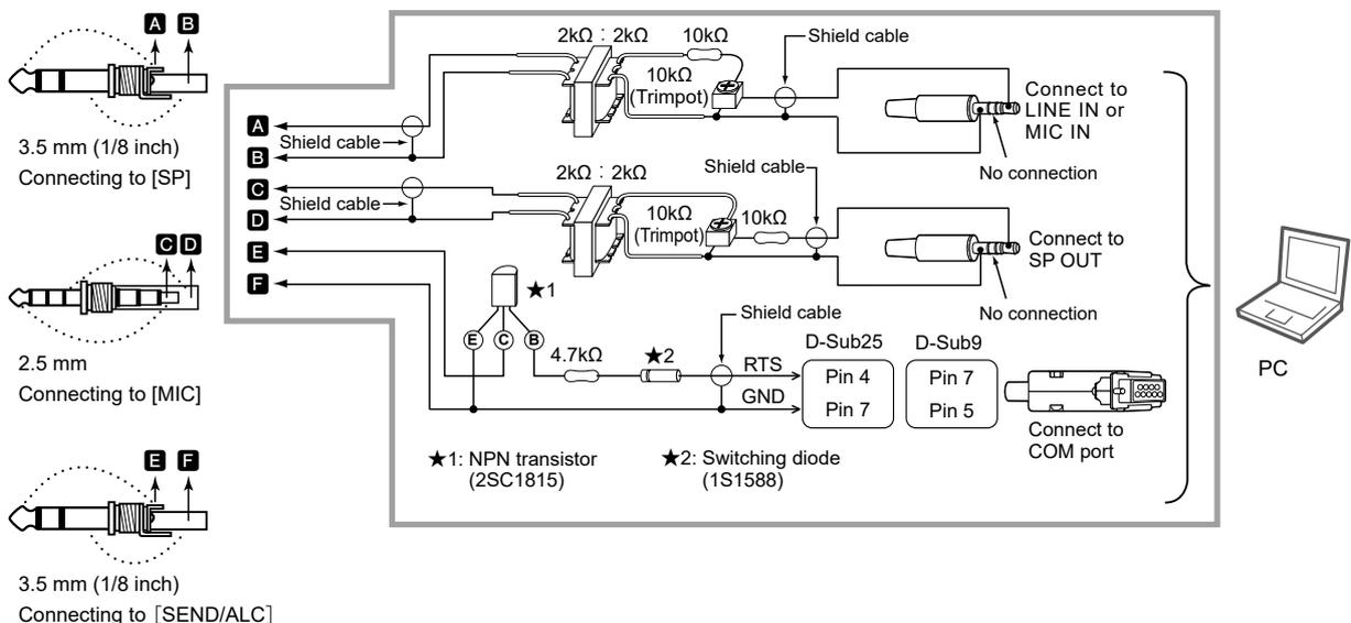
**TIP:** We recommend using the SEND terminal on the [SEND] jack to change receiving and transmitting. If you use the PTT terminal on the [MIC] jack, the data may be cut off.
