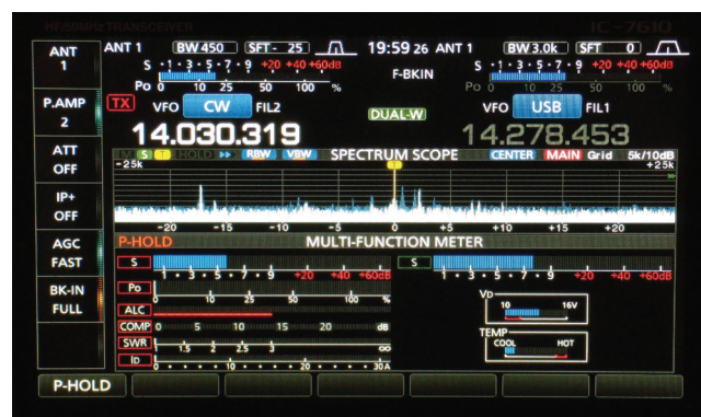
Figure 4 — A more compact bar graph of a selected meter at the top of the display allows more room for the spectrum display, or all meter choices can be viewed simultaneously, as shown here.
