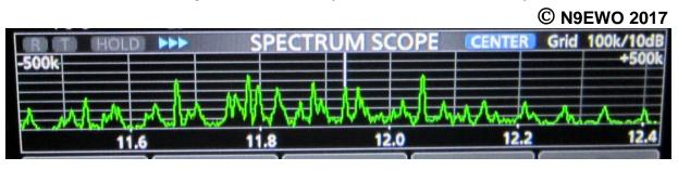
Improved "Spectrum Scope" settings for the ICOM IC-7300. Waterfall not selected in standard screen due to the limited space available (much more useful in EXPD Screen, "Small" Size). Adjusting the "Center Type Display" to "Carrier Point Center (ABS Freq)", will give for proper "centered" showing of AM signals on the scope and will also show frequency on the bottom scale in "center" mode which is a very desirable setting.
