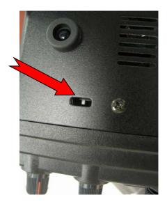
3. Connect the serial straight through programming cable, DB9F to DB9F, connector to the serial port COM1 in the back of your computer. Plug the DB9F connector to the CAT connector on the FT-450D.
