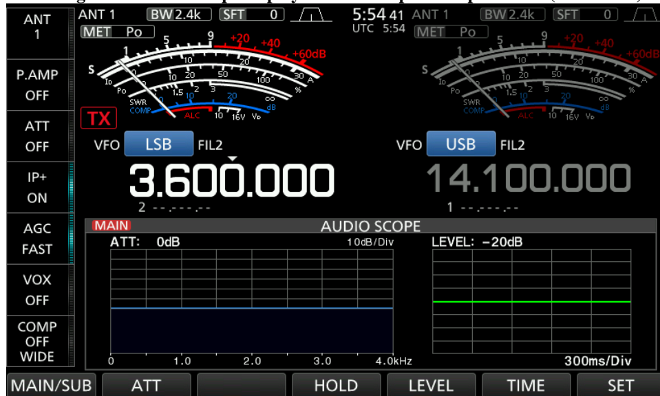
Figure 4c: Audio scope display for AGC impulse response test (NB/NR on).
