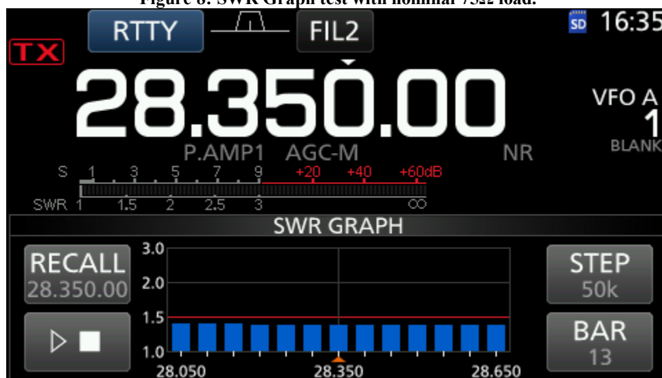
Figure 8: SWR Graph test with nominal 75Ω load.
