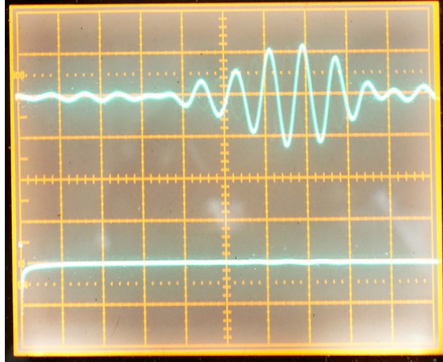
Figure 7: RX latency, 250 Hz SOFT CW filter. 2 ms/div.
